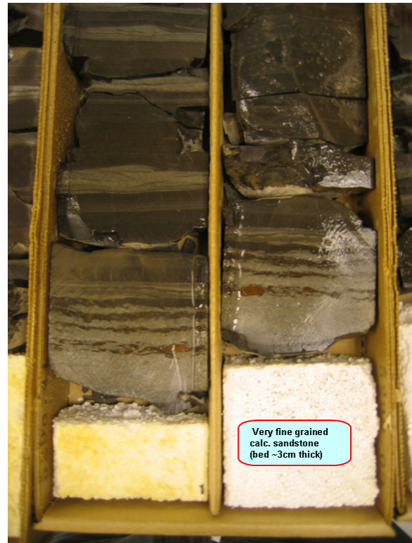
Figure 83. Tantallon M-41: Core #3 (~ 5300 m), close up of sandy intervals.
