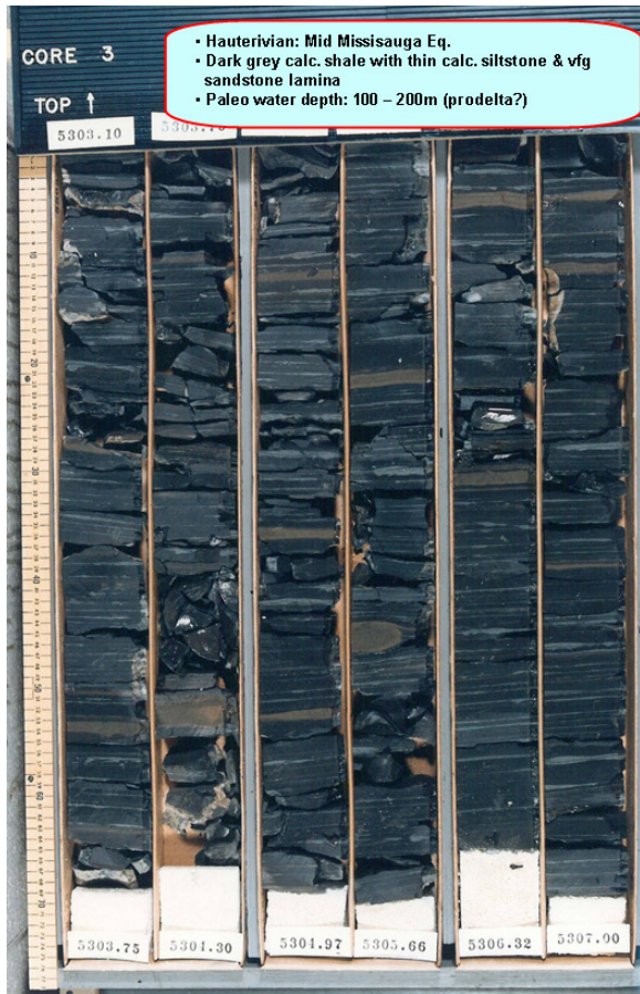
Figure 82. Tantallon M-41: Core #3 (5294.0 – 5313.0 m, 16.3 m recovered).
