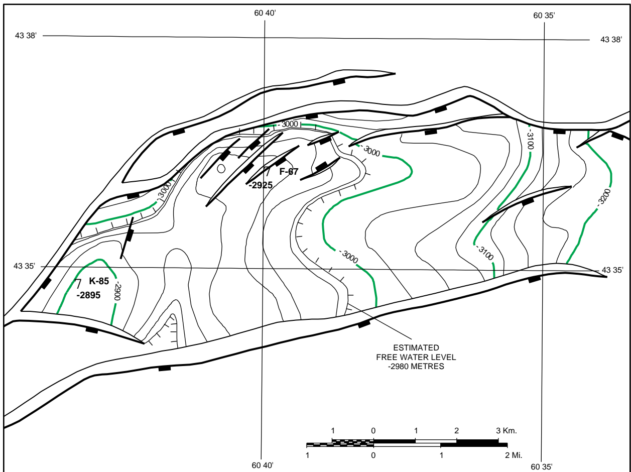
Figure 2.2.6.2.1(a): Alma - Top B Sand, Depth Structure Map Contour Interval: 25 metres
